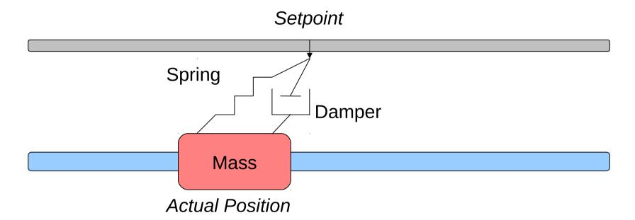
P is the spring constant, D is the degree of damping stiffness
