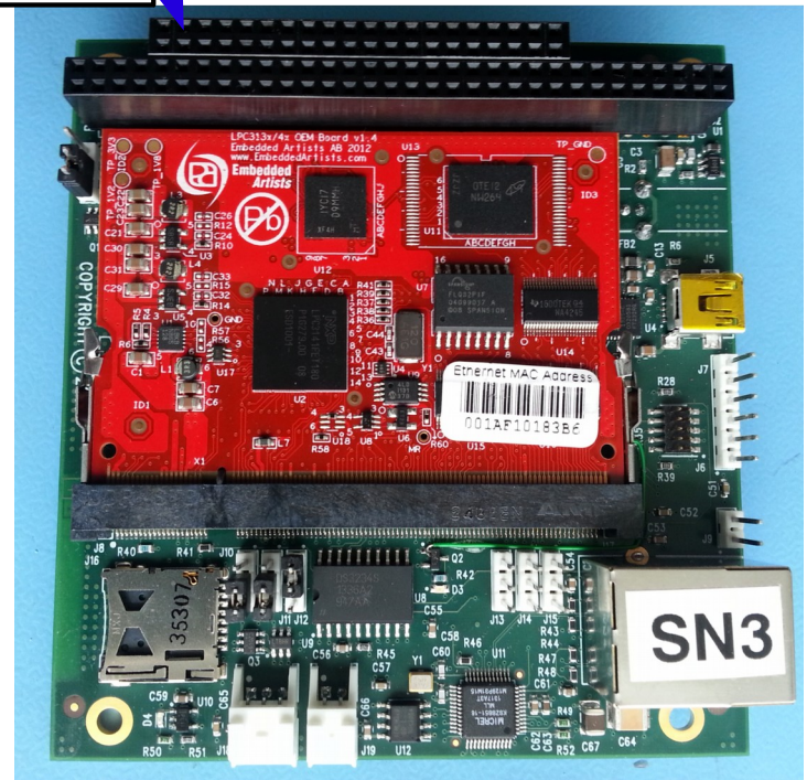
Embedded Artists LPC3141 270Mhz ARM9 64MB RAM, 256MB NAND flash, 2.6 Kernel
